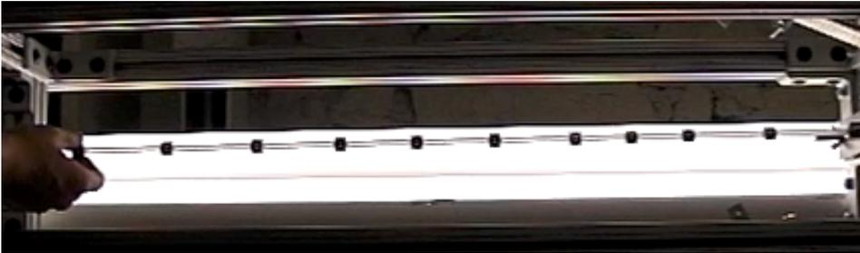
Fig. 3.5 Acoustic wave in the one-dimensional chain is created an impulse input to the system
